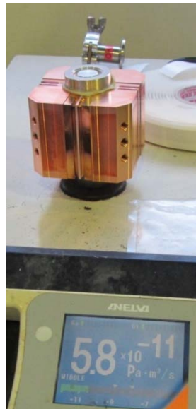
3. Vacuum leak test just after the EBW
